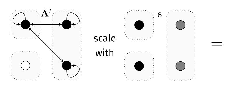
4. The final count c is  $\sqrt{\sum_{i,j} C_{ij}}$ . The square root undoes the squaring from taking the outer product (note:  $(\sum_{i} a_i)^2 = \sum_{i,j} A_{ij}$ ). The count is one-hot encoded<sup>3</sup> and scaled with a learned confidence about the prediction. The resulting feature vector is fed into the answer classifier.
