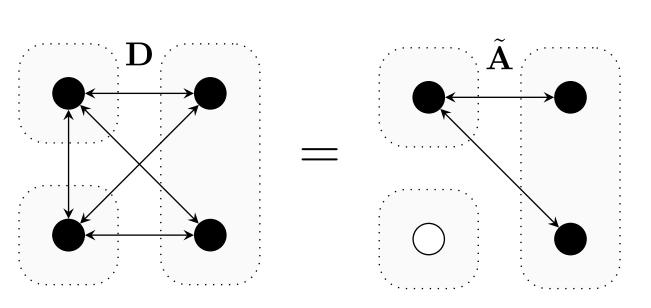
3. Inter-object deduplication: Compute similarity vector s from  $\hat{A}$  that measures for each node the number of nodes with a similar neighbourhood. Add self-loops back to  $\tilde{A}$  to obtain  $\tilde{A}'$  and scale with s to obtain the final count matrix C. Under a sum, C is equivalent to a graph that has no more than proposal per object.
