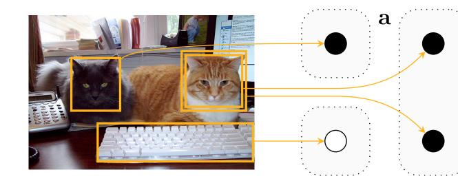
2. Intra-object deduplication: Mask away edges between overlapping proposals of A by multiplying with distance matrix D to obtain  $\tilde{A}$ . Two nodes in D are connected if their corresponding proposals do not overlap.
